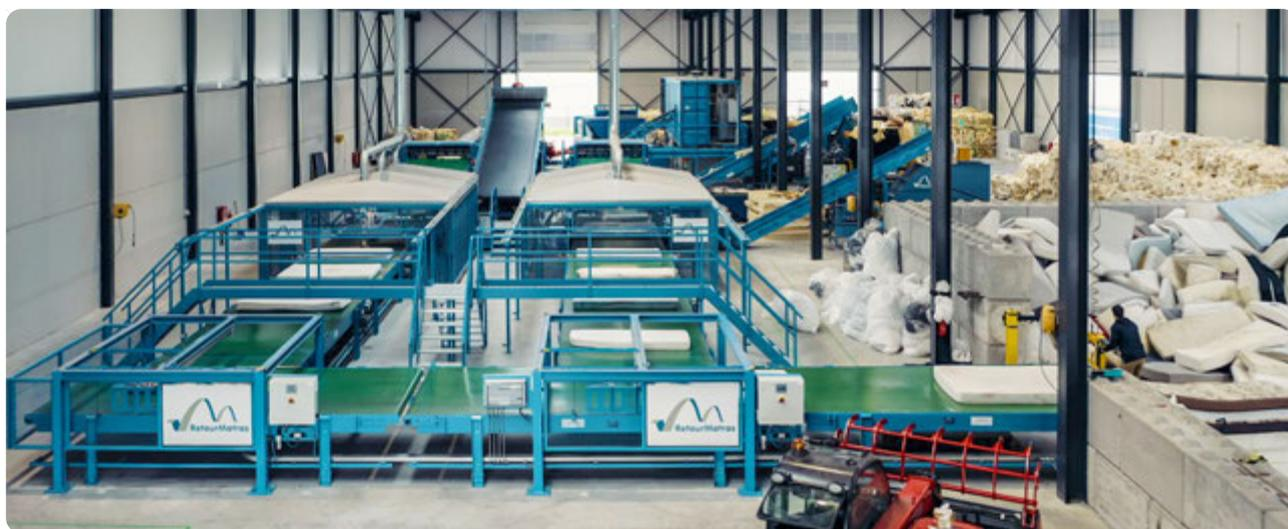
The metal springs are reused in the steel industry and fully recycled for a wide variety of uses. The foam, which comprises the majority of the mattress, is shredded, steamed and compressed. The resulting material can then be used, for example, for insulation. This is an effective form of downcycling. By following this disposal and dismantling process, we limit CO<sub>2</sub> emissions that result from burning mattresses, and the majority of the remaining materials are reused.
